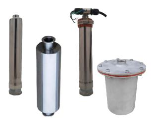
The AOD series - Ozone Destructors units utilizes a thermal-catalytic method to safe catalize ozone to oxygen reliable with no consumables. All the models uses Carulite 200 as destruct media. It is a hopcalite-type using mandanese dioxide and copper oxide. Carulite is not consumed by the ozone and is a safe material that is not considered hazardous waste.
