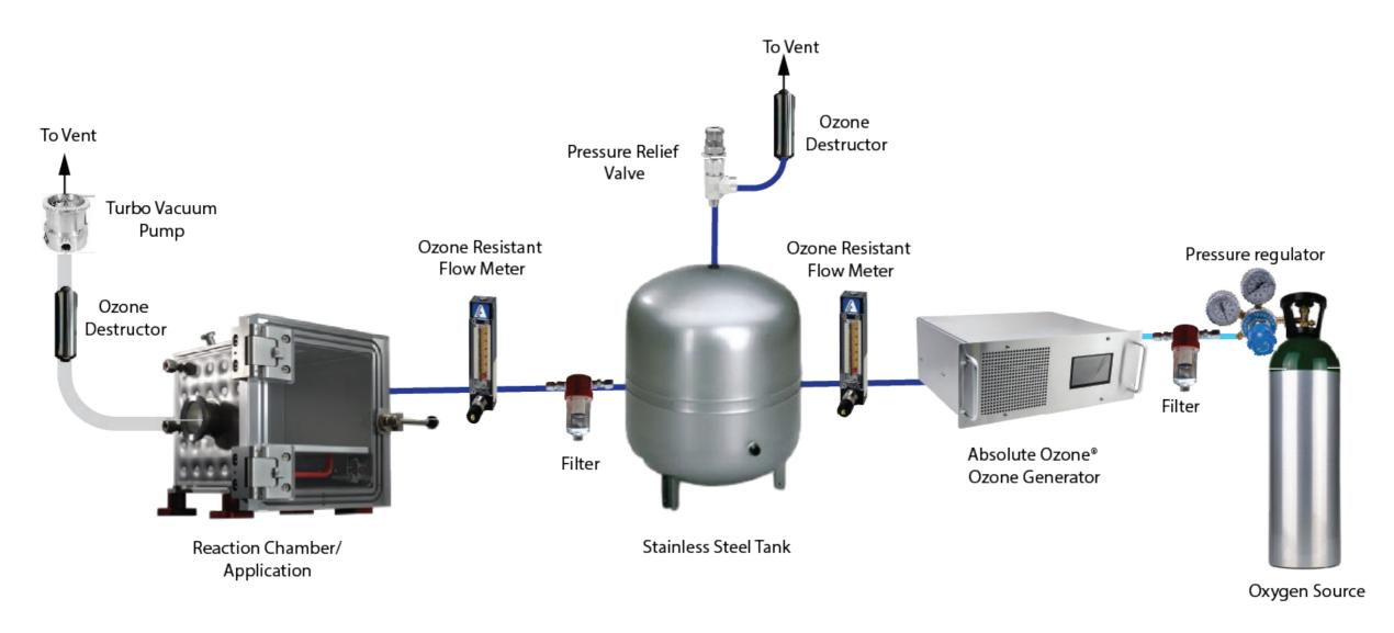
The use of an ozone generator in **SEMICONDUCTOR AND ALD** processes offers several advantages, including high reactivity, precise control over film thickness, versatility in material deposition, low-temperature processing, cost-effectiveness, environmental friendliness, reduced process steps, improved surface coverage, and compatibility with various applications. These benefits collectively contribute to the efficiency, quality, and sustainability of the ALD deposition process.
