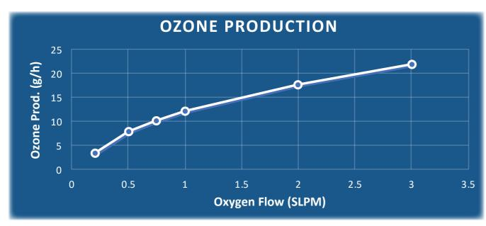
The performance is unequaled for air cooled generators. Absolute Ozone TITAN UHC reliably producing high concentration ozone **up to 22% by weight.**
