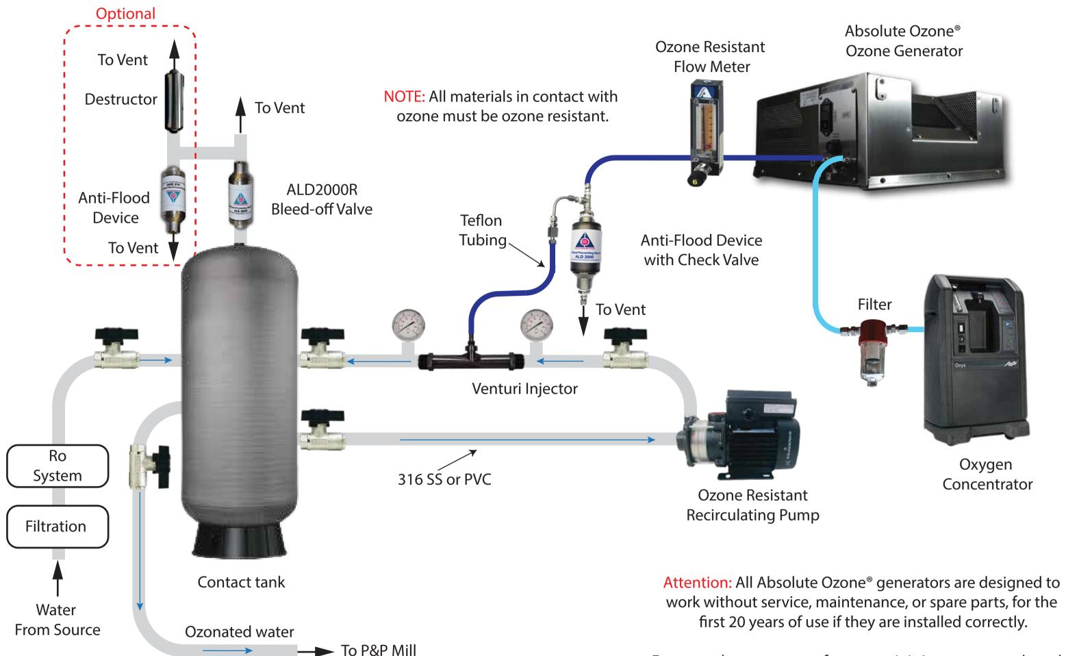
For a good generator performance, it is important to place the generator in a well-ventilated, dust free environment, and maintain the ambient temperature at 20-22°C
