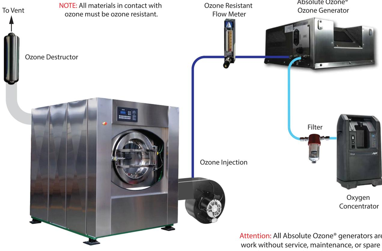
Attention: All Absolute Ozone<sup>®</sup> generators are designed to work without service, maintenance, or spare parts, for the first 20 years of use if they are installed correctly.
