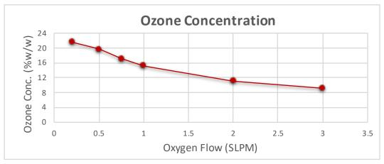
Test was performed at 20°C, Generator was ON for more than 30 min.
