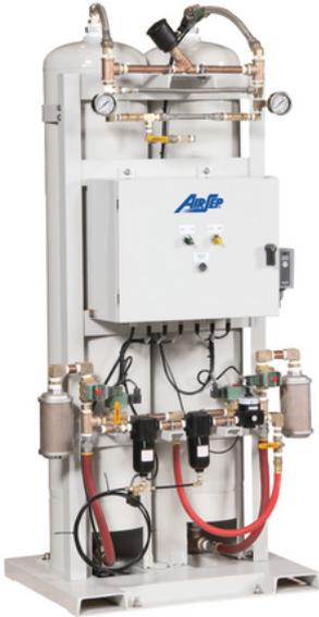
AirSep Alpha Series Oxygen Generators produce from 20 to 5,500 cubic feet of oxygen per hour at up to 95% oxygen concentration.
