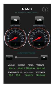
The LCD screen displays the following parameters:
