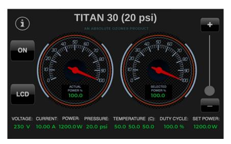
The LCD screen displays the following parameters:
