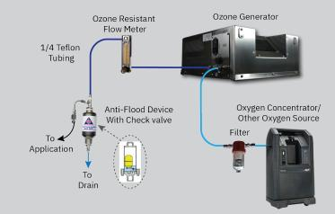
The ALD 2000 contains a stainless steel float-operated valve and hardended stainless steel seat and disc. When liquid enters the drainer, the float rises opening the valve allows liquid to drain out from pressurized ozone systems without the loss of pressured gas.
