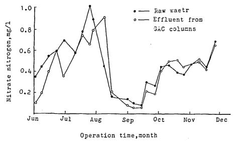
Figure 12. Evolution of nitrate nitrogen through GAC columns.
