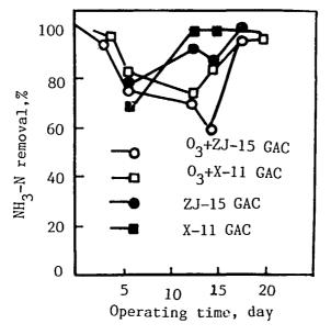
Figure 5. NH<sub>3</sub>-N removal curves for "O<sub>3</sub>-BAC" and "BAC" processes.
