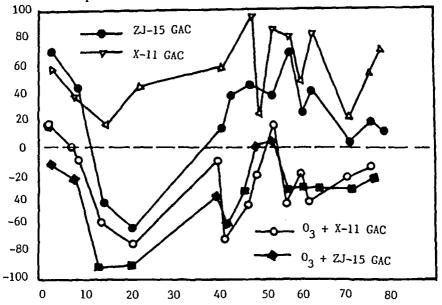
Figure 7. Nitrate nitrogen removal curves for the "O<sub>3</sub>-BAC" and "BAC" processes.
