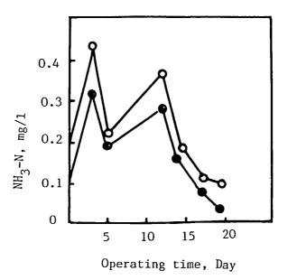
Figure 4. NH<sub>3</sub>-N content curves for raw water (lower) and ozonated water (upper).
