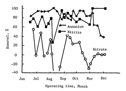
Figure 13. Removal efficiencies for NH<sub>3</sub>-N, NO<sub>2</sub>-N, and NO<sub>3</sub>-N.
